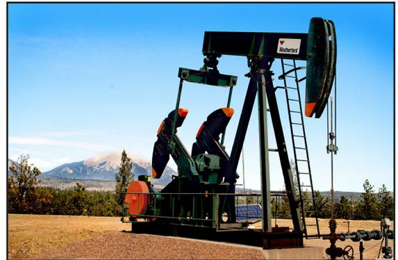
**MasterDrive** offers a complete line of stock and custom made solutions for v-belt drives and their components used in the oil and gas industries. We offer v-belt drives for all types of Artificial Lift Systems including RRL and Top Drive PCP systems.
