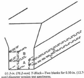
FIG. 4 Sectioning Procedure for Y-Blocks
