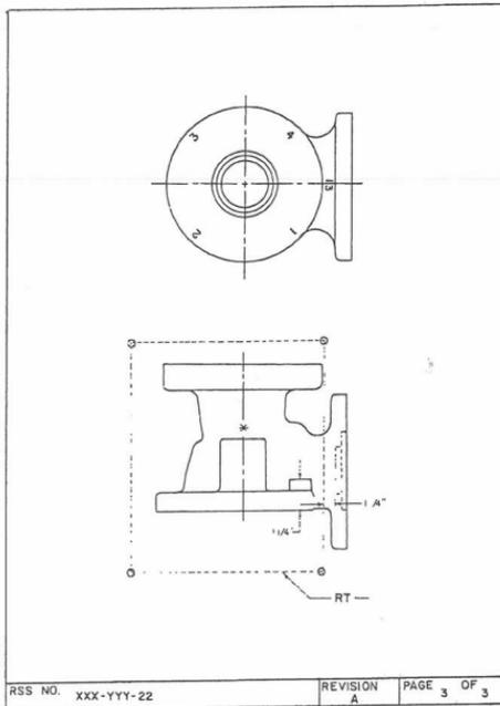
FIG. X1.3 Samples of Radiographic Standard Shooting Sketches (RSS)
