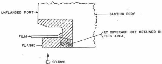
NOTE 1—This alignment provides a suitable alternative when other casting appendages (bosses, flanges, etc.) project into the radiation path as illustrated in Fig. X2.2 when this alignment is used, additional losses in coverage (as opposed to Fig. X2.1) should be expected and noted accordingly on the applicable RSS.
