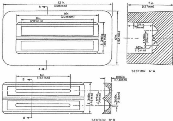
FIG. 3 Mold for Modified Keel Block
