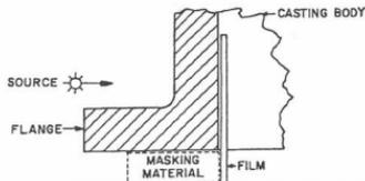
Note 1—This alignment is permissible if the radiation source energy and film multi-load capabilities are sufficient to afford compliance with the technique requirements stipulated herein. This alignment will generally require the use of filters or masking to reduce the influence of radiation that undercuts the thicker areas and reduces overall radiographic quality.
