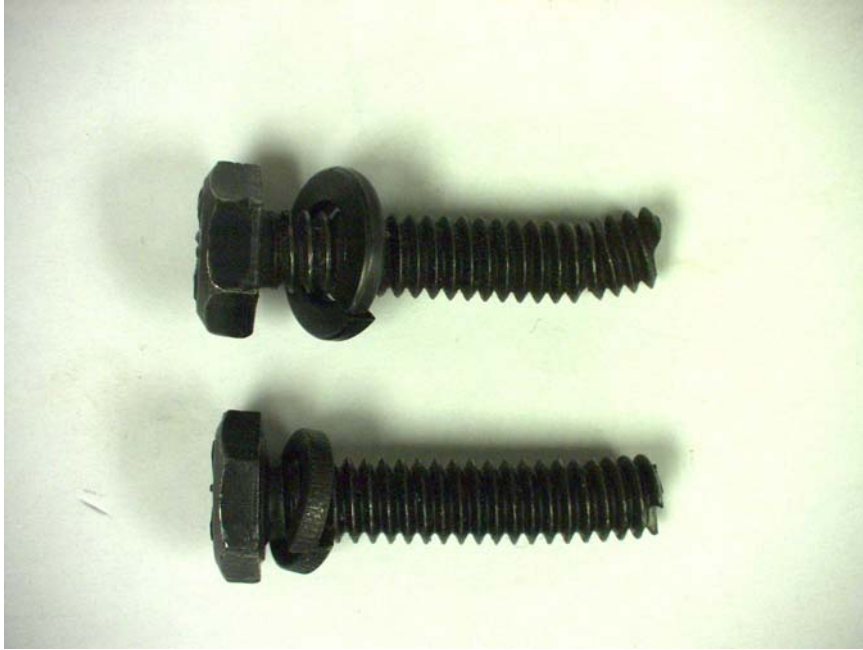
Fig. 3 - Overall view of failed cap screws is shown.
