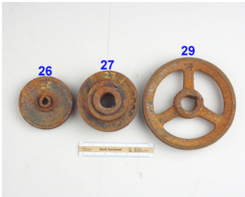
Fig. 7 - The Maurey sheaves identified as Samples 26, 27 and 29 are shown after 72 hours of salt spray testing.
