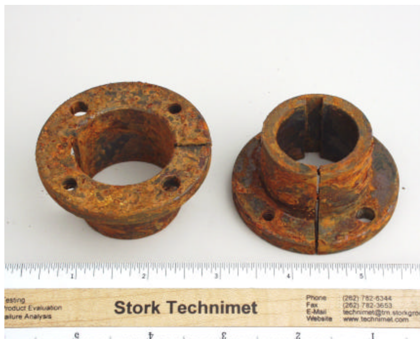
Fig. 8 - The two bushings are shown after 72 hours of salt spray testing.
