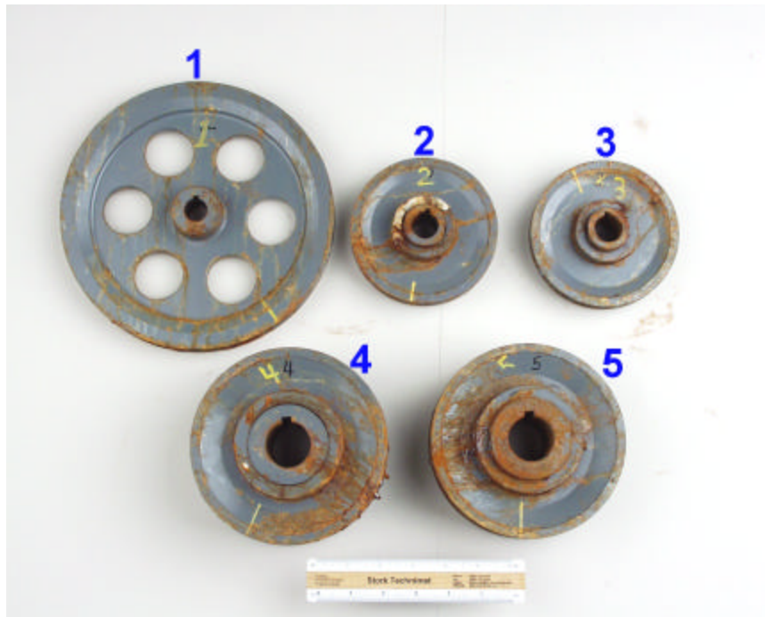
Fig. 1 - The Masterdrive sheaves identified as Samples 1-5 are shown after 72 hours of salt spray testing.
